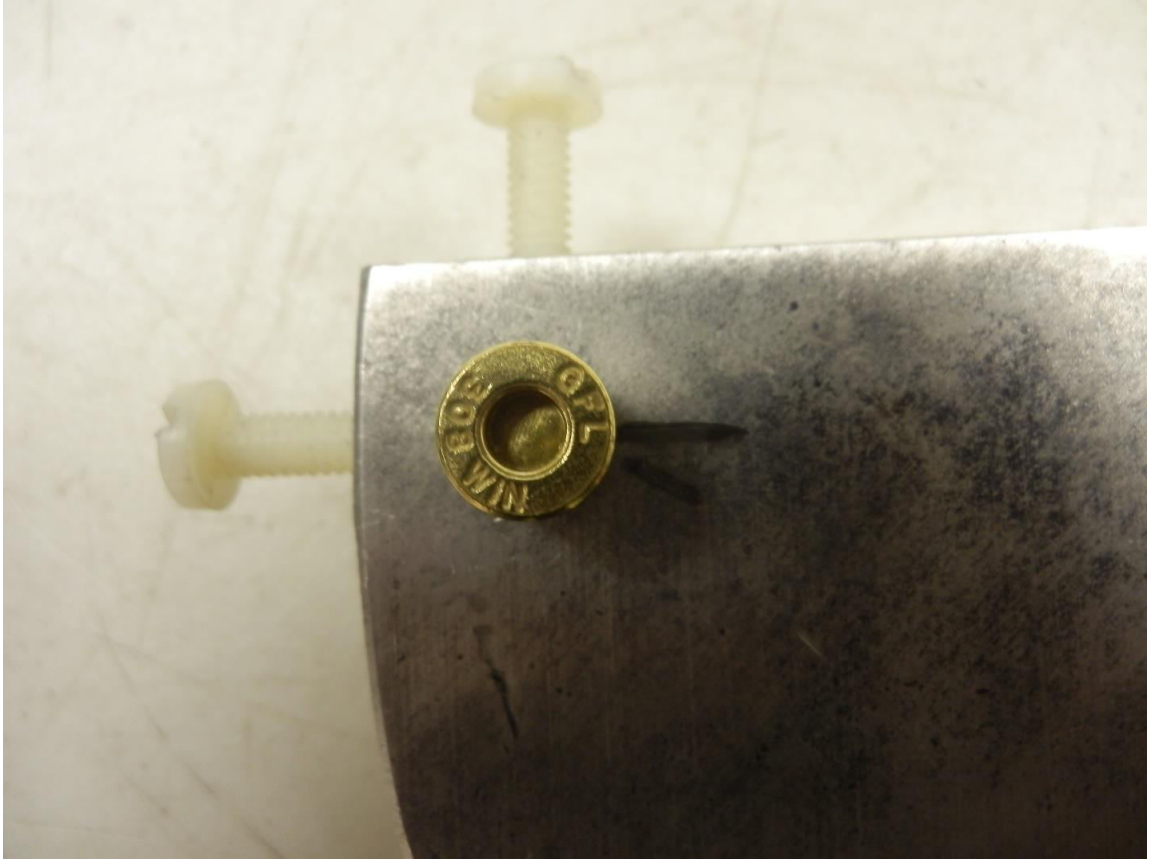
Figure 3.8. Stamped “L” in case base is lined up in case well to indicate flash hole offset direction.
