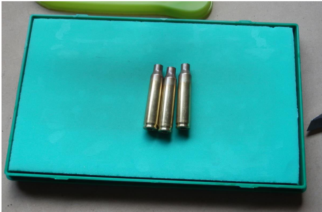
Figure 3.11. .223 cases on grease pad.
