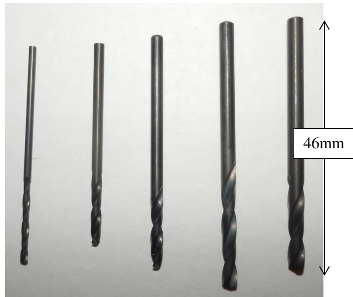
Figure 3.3. Left to right, 1.4mm, 2.0mm, 2.4mm, 2.8mm, 3.0mm drill bits used for flash hole drilling.
