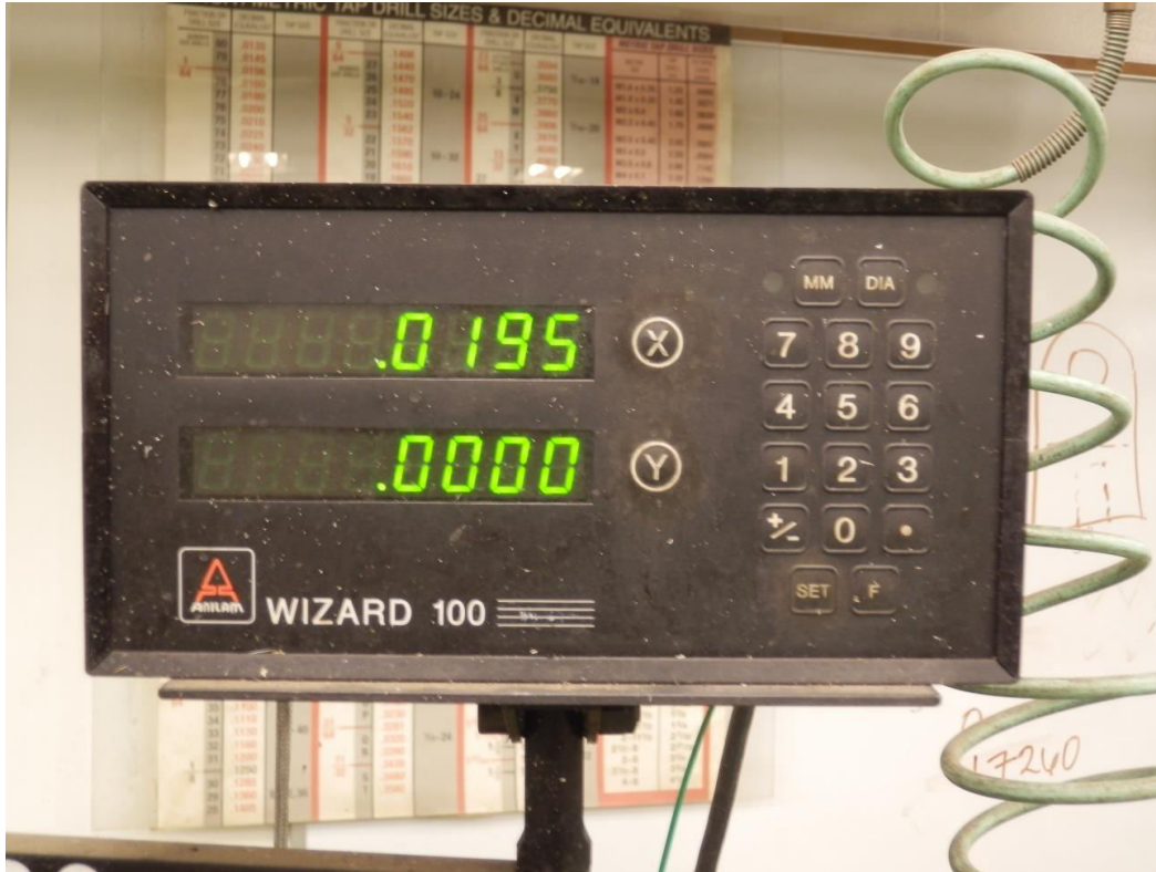
Figure 3.7. Drill offset 0.0195in (0.5mm).
