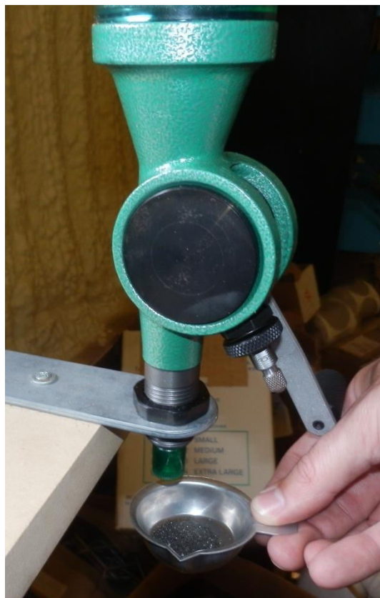
Figure 3.16. Powder dispenser and pan.
