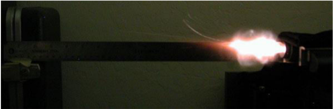
Figure 2.3. Lapua Palma case, 0.062" Flash Hole, Remington 7.5 Primer. (7)
